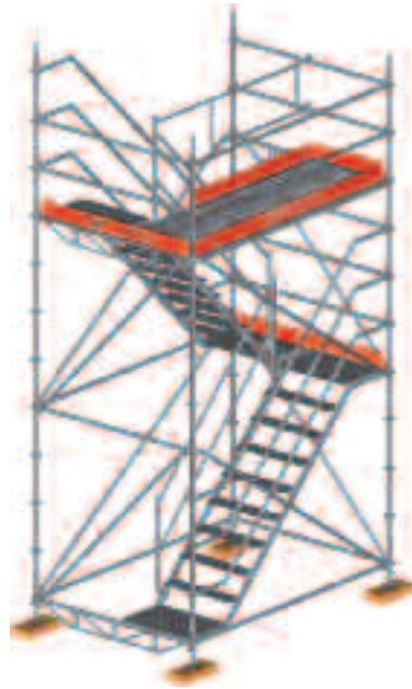
Staircase with exit on top only
